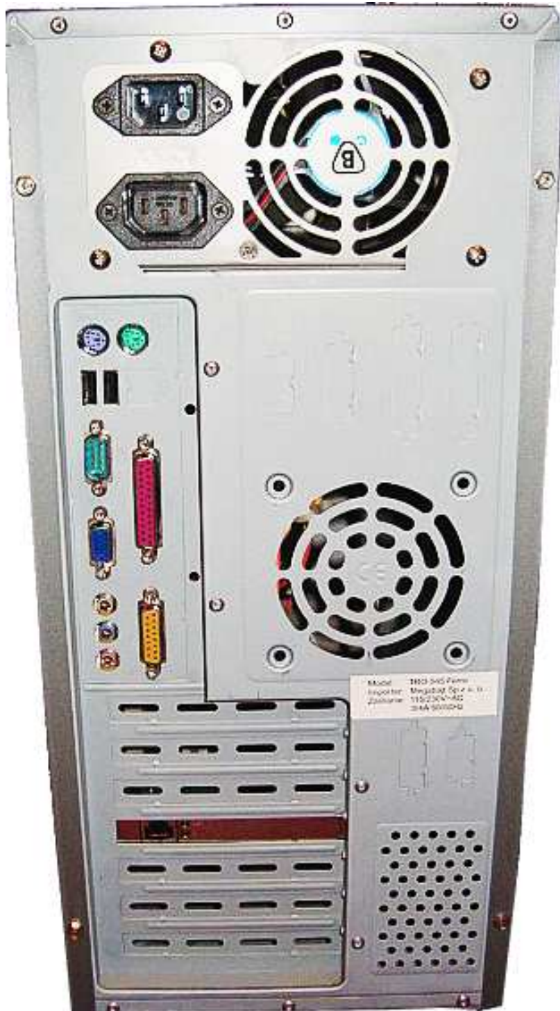
VGA, COM, PS/2, LPT, Power, USB, Game/MIDI, Audio IN/OUT, Mikrofon
